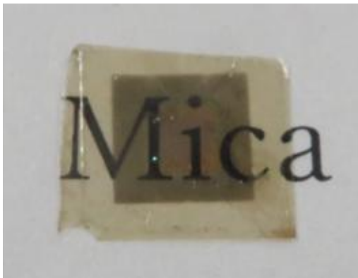
Fig.1 Photograph of BST/SRO/CFO/mica flexible structure.
